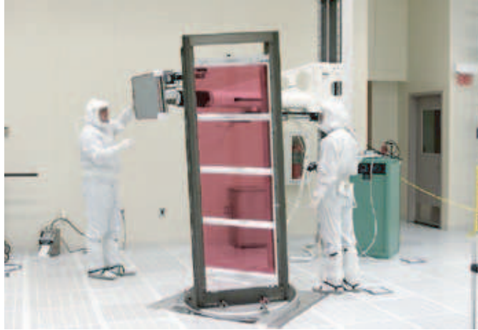
Figure 3.3: Laser Glass Assemblies for the Amplifiers
