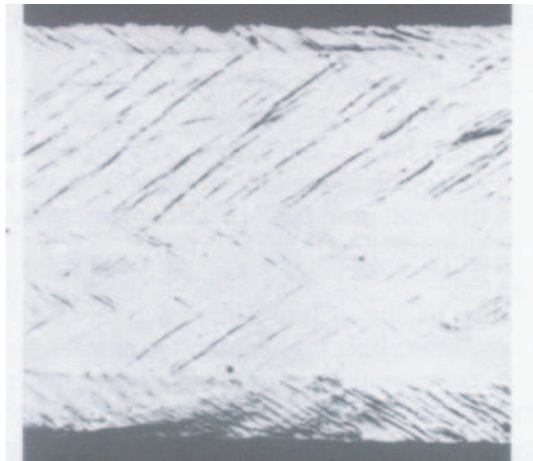
Figure 2.5: An optical micrograph of shear bands developed in plane strain rolling of a polycrystalline aluminum -4.75%wt copper alloy [20]
