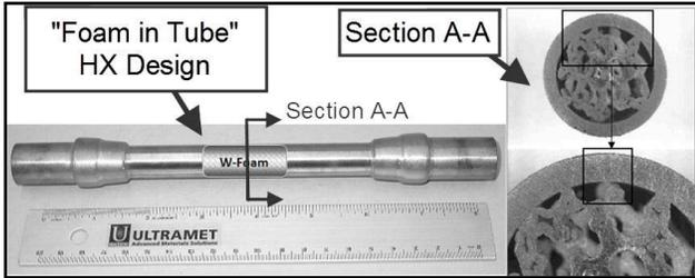
Fig. 1. Overall view (left) and section view (right) of "Foam in Tube" HX design, showing details of the CVD bond between the W-foam and tube wall (Section A-A).
