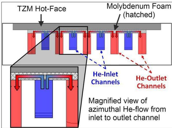
Fig. 6. Section view showing the azimuthal helium-flow.
