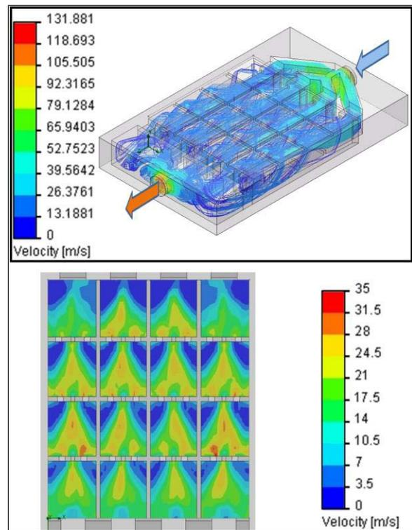
Fig. 7. CFD analysis for an early flat-plate HX concept (top) velocity streamlines and (bottom) He-velocity below heated surface [note: print copy is b&w, but color online].
