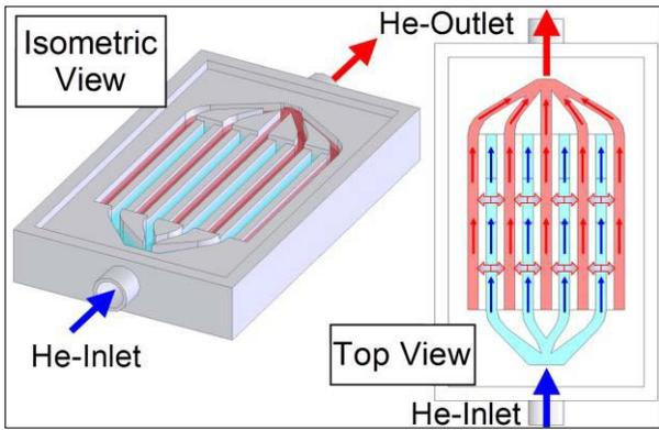
Fig. 5. Isometric view (left) and top view (right) of the HX box [note: print copy is b&w, but color online].
