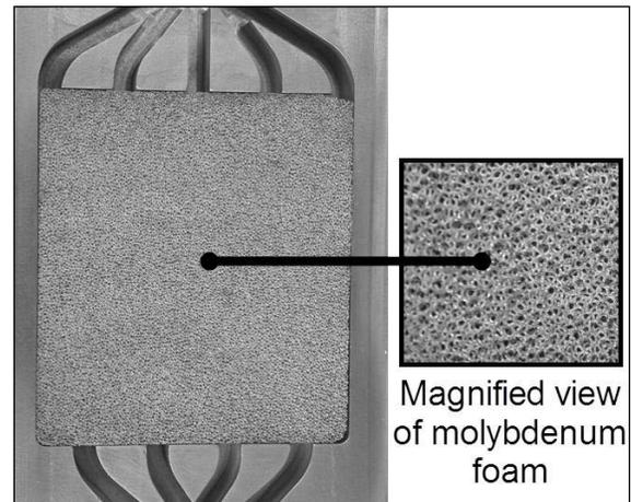
Fig. 11. Photos of the molybdenum primary structure with molybdenum foam recessed over the slotted area.
