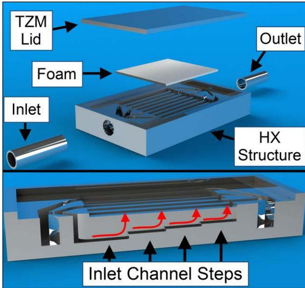
Fig. 8. Exploded view of HX prototype (top), and section view (bottom) of inlet channel steps for redirecting helium flow [note: print copy is b&w, but color online].
