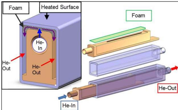
Fig. 2. Cross-sectional (left) and exploded (right) view of "azimuthal He-Flow through Foam in Tube" HX design concept.<sup>8</sup>
