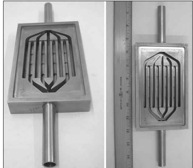
Fig. 10. Photos of the slotted molybdenum primary structure, including inlet/outlet molybdenum tubes.
