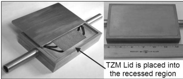
Fig. 12. Photos of foam-based HX with TZM lid partially in place (left) and with lid in place (right).
