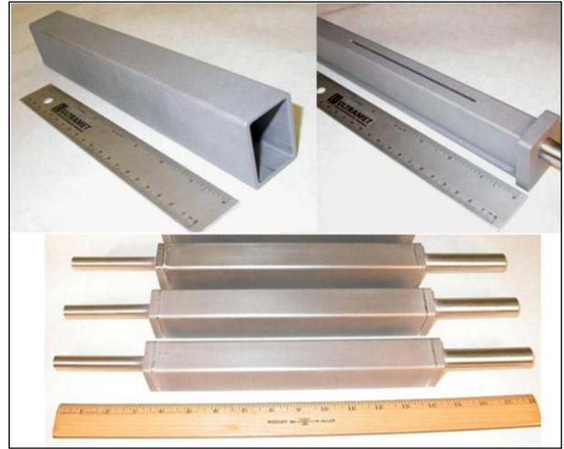
Fig. 3. Fabricated single channel "azimuthal He-Flow through Foam in Tube" HX.<sup>8</sup>
