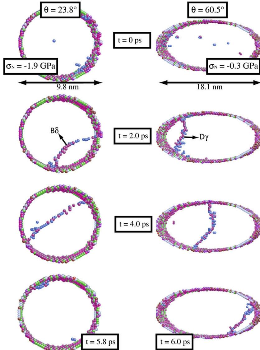
Fig. 8. Diagram showing the twin boundary migration mechanism for two characteristic compression simulations. Atoms are colored according to their coordination number, with those having 12 nearest neighbors removed. This visualization shows a slice of the pillar isolating only a few planes above and below the twin plane where the yielding event occurred. Atomic positions are the result of averaging over 50 time steps (0.1 ps)
