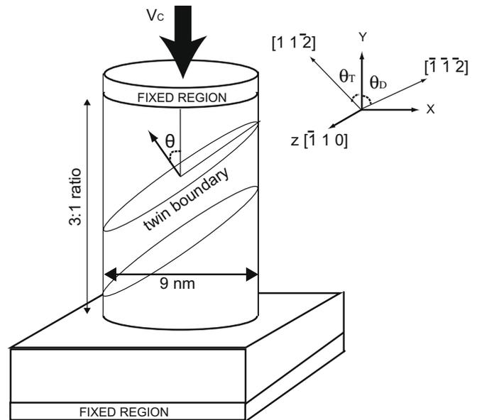
Fig. 1. Schematic of the nanopillar geometry. The two sections labeled “fixed region” are atoms which are constrained either to rigid body motion (top), or totally constrained (bottom).  $v_c$  is the rigid body velocity imposed on the upper region. The prismatic block at the bottom has periodic boundaries, while the cylindrical surface is a free boundary.
