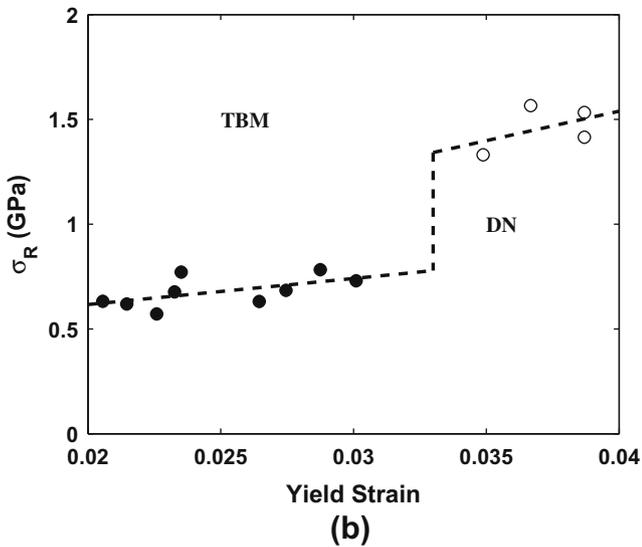
Fig. 4. (a) The normal stress,  $\langle\sigma_N\rangle$ , and (b) the critical resolved shear stress,  $\langle\sigma_R\rangle$ , plotted as a function of the yield strain for twinned copper nanopillars under compression. A clear bifurcation in the yield mechanisms takes place around a strain of 3.3%. The black dots indicate yielding by twin boundary migration and the white dots indicate yielding by dislocation nucleation.
