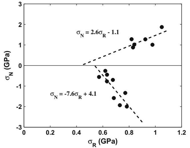
Fig. 5. Yield locus for reversible plasticity shown as the normal stress,  $\langle\sigma_N\rangle$  plotted as a function of the critical resolved shear stress,  $\langle\sigma_R\rangle$  for twinned nanopillars in tension (positive  $\langle\sigma_N\rangle$ ) and in compression (negative  $\langle\sigma_N\rangle$ ).
