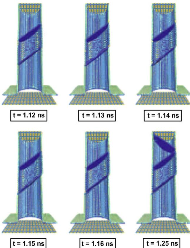
Fig. 7. Time sequence of the yielding of nanopillar tension at  $\theta = 35.3^\circ$ . All other conditions are the same as in Fig. 6.
