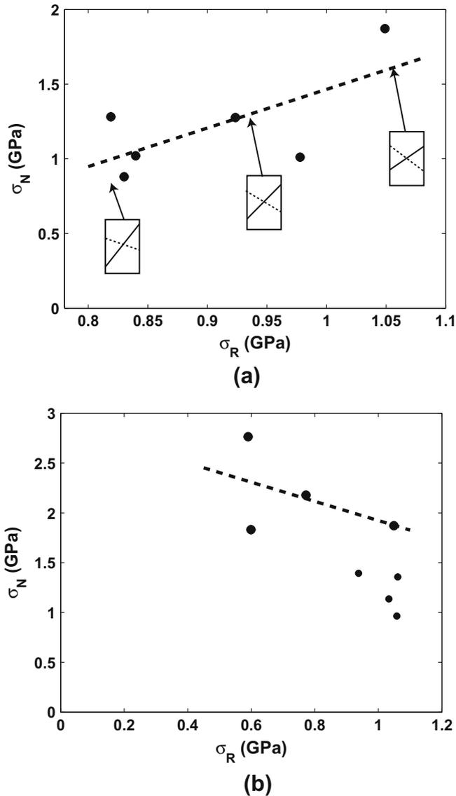
Fig. 2. “Yield locus” in the twinned nanopillar under tension shown as a linear relationship between the normal stress,  $\langle\sigma_N\rangle$  and the resolved shear stress,  $\langle\sigma_R\rangle$ . (a) The regime of exclusively twin migration behavior (reversible plasticity) and (b) the regime of irreversible plasticity resulting from mixed behavior, where either twin migration (large black circles) or dislocation nucleation (small black circles) from the surface is indicated.
