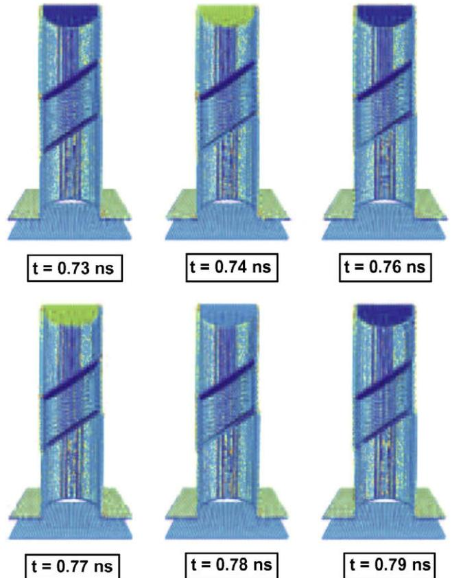
Fig. 6. Time sequence of the yielding of nanopillar compression at  $\theta = 35.3^\circ$ . Atoms are labeled according to their centrosymmetry parameter. The front half of the nanopillar has been cut away for the purpose of this visualization in order to reveal the twinned nanostructure within. The atomic positions are averaged over 5000 time steps (10 ps) to remove noise due to thermal vibrations.
