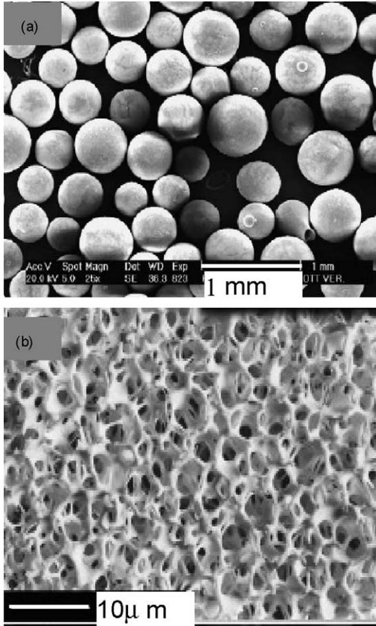
Fig. 3. Samples of (a)  $\text{Li}_3\text{SiO}_4$  pebbles and (b)  $\text{Al}_2\text{O}_3$  foam [1,21].
