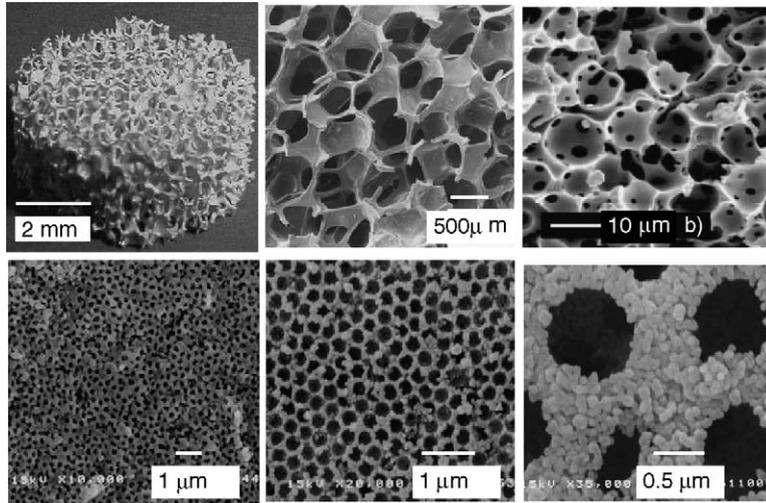
Fig. 1. Ceramic foam examples; (a) TiO<sub>2</sub> foam: positive replicated of polyurethane foam [19]; (b) pyrolyzed ceramic SiC–Si<sub>3</sub>N<sub>4</sub> composite foam [7]; (c) micro-cellular SiOC foam using a foaming agent and pre-ceramic polymer [9]; Placeholder techniques, SEM of macro-porous ceramic material prepared using suspended ceramic nano-particles with polymer spheres: (d) γ-Al<sub>2</sub>O<sub>3</sub>, (e) TiO<sub>2</sub>, (f) 3Y-TZP [20].
