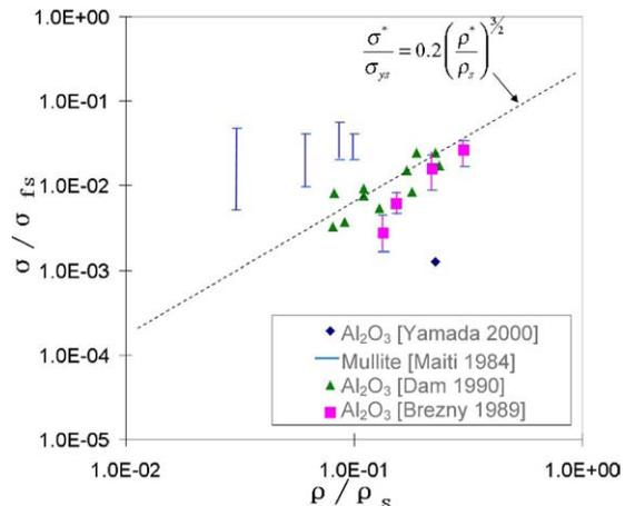
Fig. 2. Variation of relative crushing strength as a function of relative ceramic foam density (dotted line is based on alumina solid fracture strength) [11].
