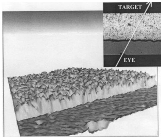
Fig. 4. An image drape of the 50/50 wt% ZrO<sub>2</sub>/Al<sub>2</sub>O<sub>3</sub> composite coating produced representing the surface morphology of the coating in terms of pixel intensity.
