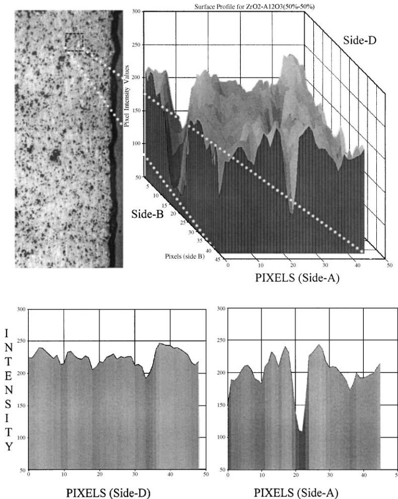
Fig. 5. Surface profile analysis of the 50/50 wt%  $ZrO_2/Al_2O_3$  composite coating.
