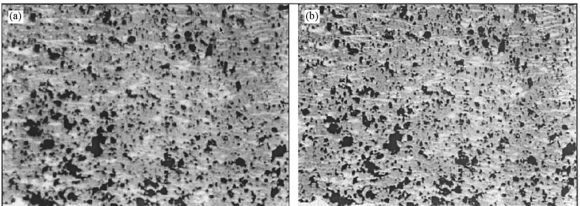
Fig. 2. Microphotograph of a coating produced with a 50/50 wt%  $\text{ZrO}_2/\text{Al}_2\text{O}_3$  powder mixture: (a) raw data, (b) image enhanced ( $200\times$  magnification).
