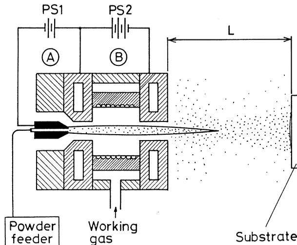
Fig. 1. Schematic diagram of gas-tunnel-type plasma torch: (A) conventional plasma torch, (B) vortex-stabilized plasma torch. PS-1, PS-2; power supplies.
