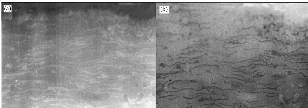
Fig. 3. Microphotograph of a coating produced with a 50/50 wt%  $\text{ZrO}_2/\text{Al}_2\text{O}_3$  powder mixture: (a) raw data, (b) image enhanced ( $500\times$  magnification).
