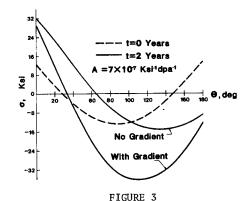
effect of damage gradient on stress distribution
