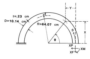
FIGURE 1 configuration of pipe model
