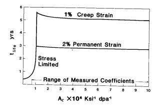
FIGURE 5 end of life for assumed failure criteria
